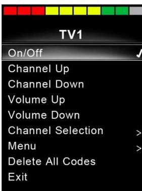
Figure 29 – IR code stored for 'On/Off' command.
