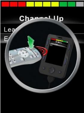
Figure 33 – 'Learn Code' process screen, awaiting IR transmission from remote.
