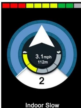
Figure 42 – Single switch scanner drive mode.
